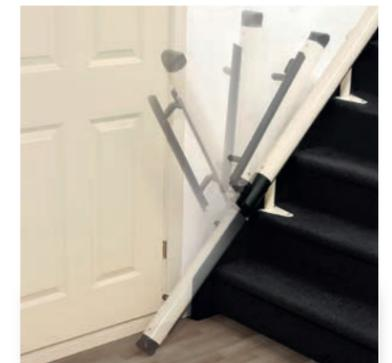
The Freecurve can be combined with a **powered hinge** or **drop nose** option to prevent the track from obstructing a doorway at the base of the stairs.
